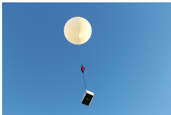
Figure 1. A meteorological balloon carrying infrasound sensors in a PolarTech insulated shipping container in 2015. The parachute is visible between the box and the balloon. The Skyfall set-up is very similar to the one shown and described here.
